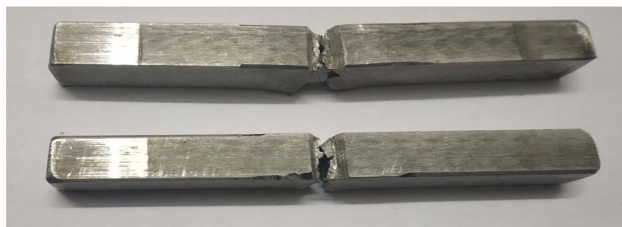
Fig. 7 Specimen subjected to Charpy V-notch test
