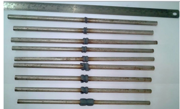
Fig. 3 Sample joints formed during friction welding
