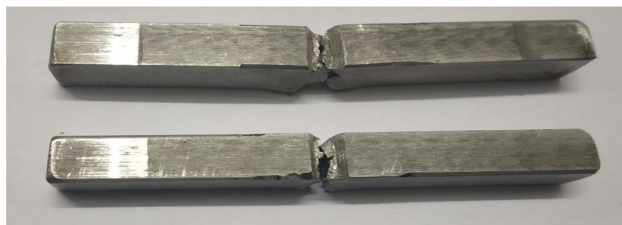
Fig. 7 Specimen subjected to Charpy V-notch test
