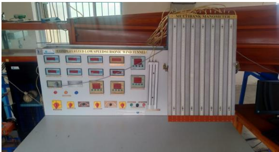
Fig. 5. Wind tunnel control panel and Muti-Bank
