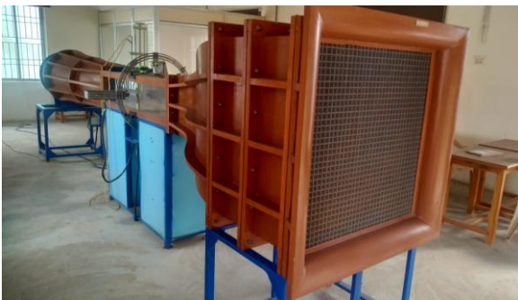
Fig. 2. Honeycomb and settling chamber
