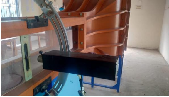
Fig. 9. Strain Gauge Balance
