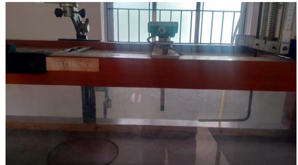
Fig. 8. Pitot-Static tube and Hotwire anemometer
