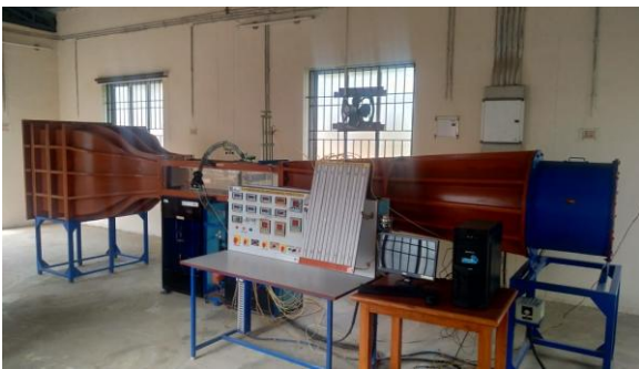
Fig. 1. Low-speed Subsonic open circuit and suction type wind tunnel in TNPESU
