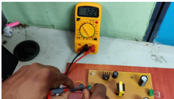
Fig 4. Input voltage of 12V
